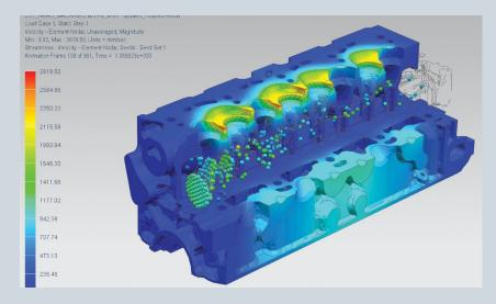
NX Advanced Flow enables you to model and simulate complex fluid flow problems through an element-based, finite volume CFD scheme used to compute 3D fluid velocity, temperature and pressure by solving the Navier-Stokes equations. Applications of NX Advanced Flow include:
